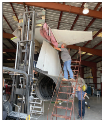
Installing horizontal stabilizer
