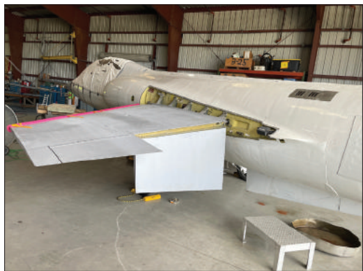
right wing installed
